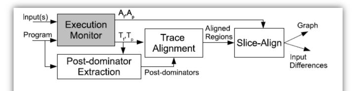
Figure 4: System architecture. The darker box was previously available.
