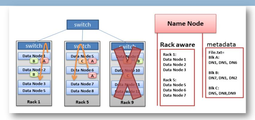
Typically, large Hadoop clusters are arranged in racks and network traffic between multiple nodes within the same rack is much more desirable than network traffic across the racks. In addition, the NameNode tries to place replicas of each block on multiple racks for improved fault tolerance.
