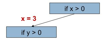
Logical operation – instrument conditionals to record inputs that caused particular branches to run
