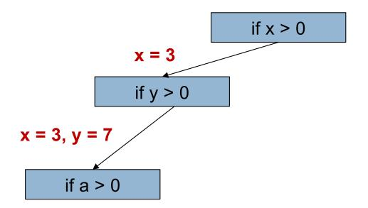
Logical operation – instrument conditionals to record inputs that caused particular branches to run
