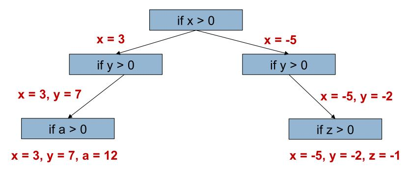
Track the branch coverage and generate inputs to explore new branches
