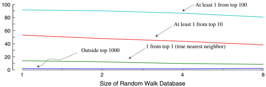
Fig. 13 The percentage of cutoffs for various rankings, for increasingly large databases with approximate search
