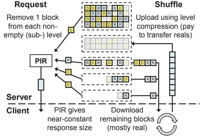
Figure 2: In OS+PIR, PIR reduces the response cost for each request to near-constant. During shuffling, only blocks remaining in each level (largely real) need be downloaded. With level compression, we need only transfer data of size equal to the uploaded reals. In all, dummy transfers are “free” — we effectively pay only to transfer real blocks.
