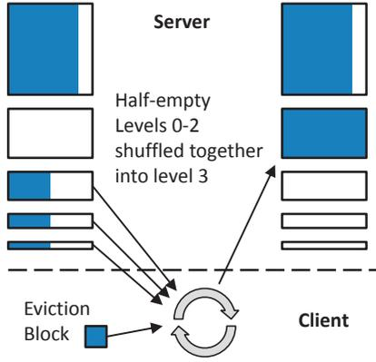
Figure 1: When shuffles cascade upward in OS, all levels to be re-shuffled are downloaded, shuffled with eviction blocks, and uploaded to a higher level.
