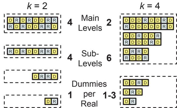
**Figure 3: Level configurations with size factors  $k = 2$  and  $k = 4$ , both with 15 real-block capacity. When shuffling, all sub-levels in a main level combine to form one new sub-level in next largest main level.  $k = 4$  configuration has fewer main levels, thus lower shuffling costs.  $k = 2$  has fewer dummies and sub-levels, thus lower disk and PIR costs.**
