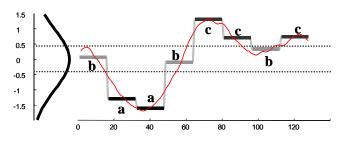
Figure 4. A real valued time series can be converted to the SAX word **baabccbc**. Note that all three possible symbols are approximately equally frequent.
