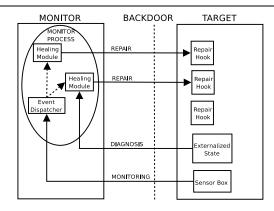
Figure 1. Software architecture for remote repair using Backdoors.
