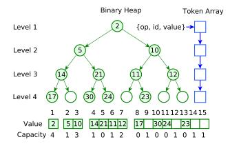
Figure 3: The P-heap data structure[23]
