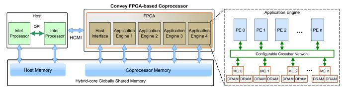
Figure 1: Overview of the Convey Hybrid-Core architecture
