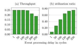
Figure 12: Effect of variation of processing delays (in cycles) on (a) throughput, (b) ratio of core utilization for 64 event processors with 256 LP and 512 initial events.
