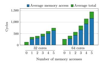
Figure 11: Effect of number/size of state memory access on event processing time
