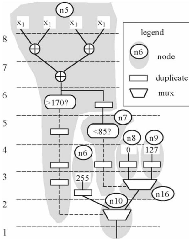
**Fig. 6** DFG of the gray scale transformation example. The numbers on the left side are the execution levels. The dashed lines carry speculators, while the solid lines carry data values. The nested if-else statements are converted into a data-flow free of control. Speculators are duplicated along the execution levels. Each execution level is an instantiation of one iteration. Notice that latches can be added between any execution levels
