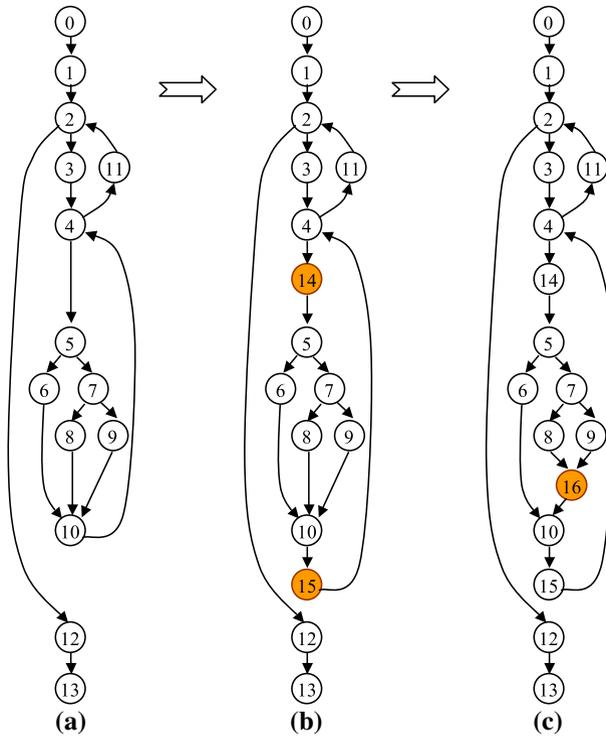
**Fig. 5** CFG of the gray scale transformation example. (a) The original CFG. (b) The CFG after pre-processing: highlighted nodes are added. Node 14 is the smart buffer node and node 15 is the memory write FIFO buffer node. (c) The CFG right before performing if-conversion. Node 16 is added to make each joint node have only two predecessor nodes
