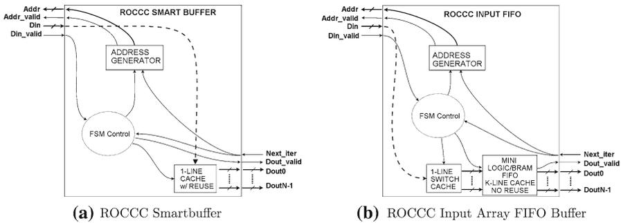
Fig. 10 Smartbuffer and input array FIFO buffer
