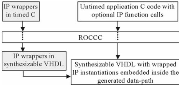
**Fig. 13** ROCCC’s workflow when IP function call present. Notice that an IP core is not necessarily a mandatory element of the main untimed application C code. The grayed out part on the left only exists when there is an IP instantiation in the source code
