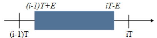
Fig. 4. Permitted sending intervals (sender's clock)
