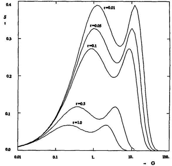
Throughput versus Traffic diagram for  $s=5$  and  $r$  varying
