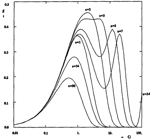
Throughput versus Traffic diagram for  $r=0.01$  and  $s$  varying
