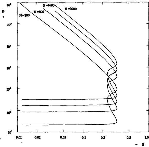
Delay versus Throughput diagram
