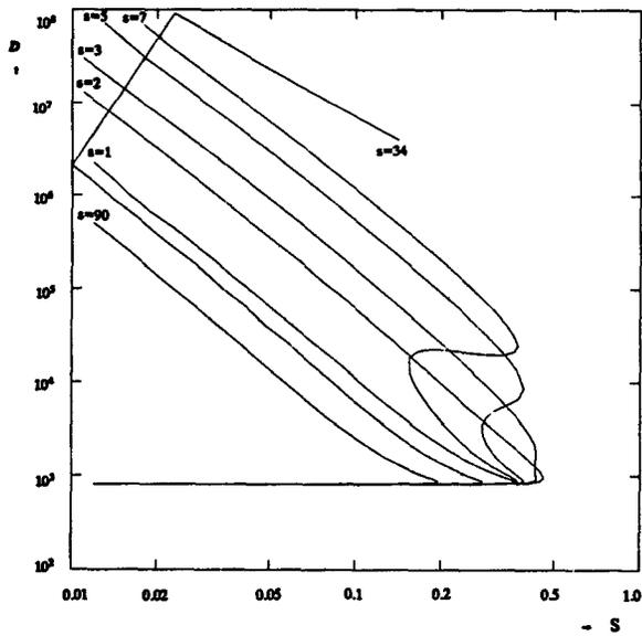
Delay versus Throughput diagram for  $r=0.01$  and  $s$  varying
