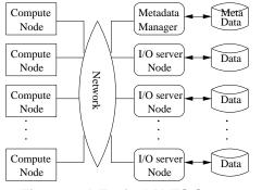
Figure 9. A Typical PVFS Setup
