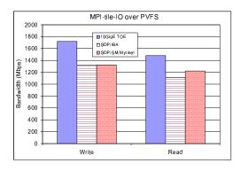
Figure 11. MPI-Tile-IO over PVFS
