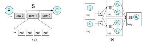
Figure 7. Data-Cutter stream abstraction and support for copies. (a) Data buffers and end-of-work markers on a stream. (b) P,F,C filter group instantiated using transparent copies.
