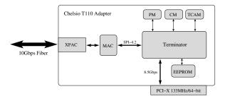
Figure 1. Chelsio T110 Adapter Architecture
