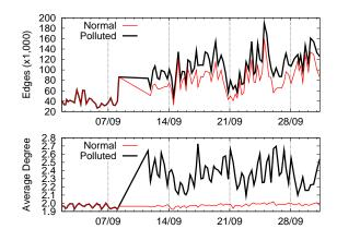
**Figure 7:** The changes in average degree (bottom) and the number of edges (top) of the Web TDG after we inject Gnutella traffic. Plots show both the values of the metrics under no pollution (normal) and after pollution (polluted).
