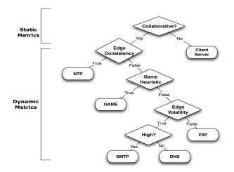
**Figure 6:** Final TDG-based classification process combining static (unary) and dynamic (binary) metrics. From top to bottom, at each level of the decision tree, the classifier selects the easier to identify application.
