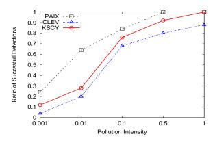
**Figure 9:** Detection rate per pollution intensity for three different backbone links.
