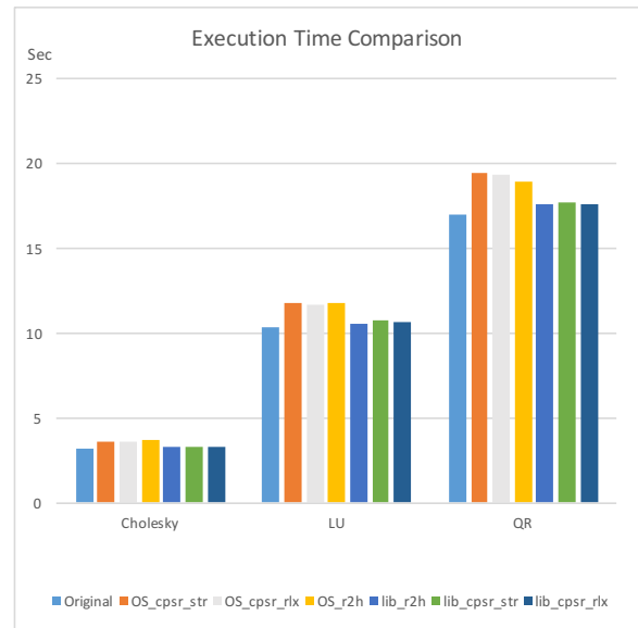
Fig. 7. Execution time of Cholesky, LU and QR factorization using several different energy saving solutions. Right two bars in each group show our results, which have similar performance than existing state-of-the-art solutions.
