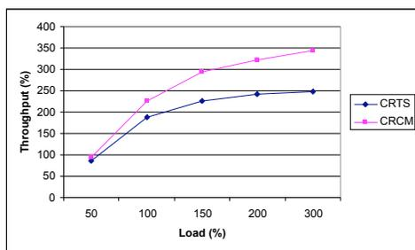
Fig. 7: Comparison between CRTS and CRCM for scenario 3
