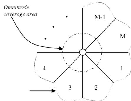
Fig. 1: The circular directional transmission
