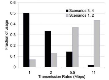
Fig. 9. With our framework, routers exploit the good channel conditions thereby using high bit rates whenever possible.
