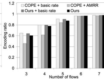
Fig. 3. The coding gain is maintained at high levels with our coding-aware rate selection module.
