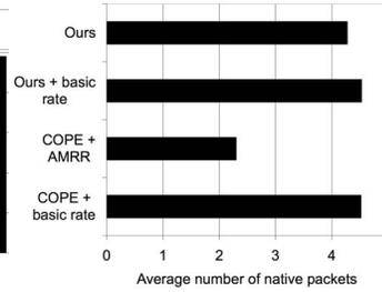
Fig. 4. Our framework enables the router to code many native packets into every new encoded packet.
