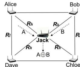
Fig. 1. Selecting high transmission rates may impede the network coding gain. Here, Alice chooses to use a high transmission rate to send her packet  $A$  to Jack. It is possible that Dave does not overhear packet  $A$ , and hence he cannot decode Jack’s  $A \oplus B$  encoded packet.
