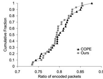
Fig. 8. Our framework achieves a very similar network coding gain as COPE, albeit the use of high bit rates.
