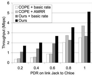
Fig. 2. Our framework provides the highest throughput gains in topologies with diverse link qualities.
