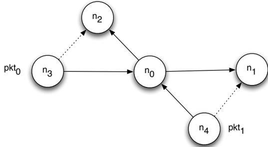
Fig. 1. Node  $n_3$  has to deliver  $pkt_0$  of flow 0 to  $n_1$ ,  $n_4$  has to deliver  $pkt_1$  of flow 1 to  $n_2$
