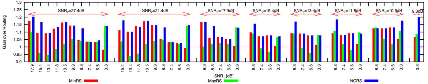
Fig. 5. Gain over routing for packets delivered to all hops for 3-node scenarios with varying SNR combinations -  $SNR_1 = \text{SNR on } n_0 \rightarrow n_1$ , and  $SNR_2 = \text{SNR on } n_0 \rightarrow n_2$ , Load = 1500pps, Maximum Gain - NCRS-MinRS: 16%, NCRS-MaxRS: 21%
