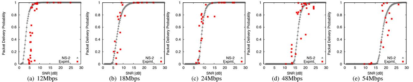
Fig. 2. Experiment vs. simulation results for 1500Byte packets
