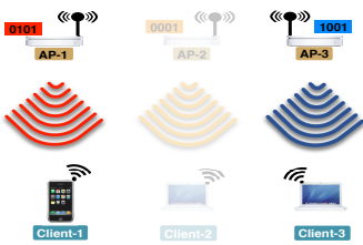
Figure 1: CSMA: (Two slot schedule: AP1,AP3 active simultaneously in slot 1, AP2 in slot 2.)
