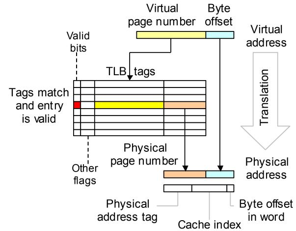
Virtual-to-physical address translation by a TLB and how the resulting physical address is used to access the cache memory.
