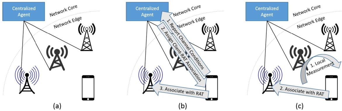
**FIGURE 2.** (a) Client with access to 3 Heterogeneous RATs; (b) Network-controlled HetNets: (1) The client reports information on its accessible RATs to the centralized agent, which (2) computes the globally optimal client-RAT association back to the client and (3) switches RATs; (c) Client-controlled HetNets: (1) The client gathers information on its accessible RATs and makes a local decision for its own client-RAT association decision and (2) switches RATs.
