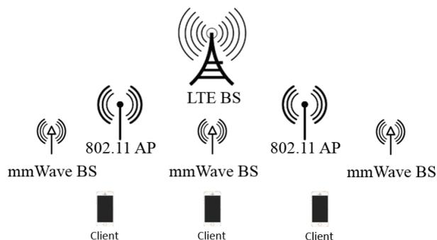
**FIGURE 1.** An example of a Heterogeneous Network with clients able to access 5G millimeter wave RATs
