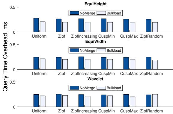
Figure 8: Query time overhead results for the the case when a dataset is bulkloaded, creating a single LSM component, vs. a workload with the NoMerge policy, creating a maximum number of components.
