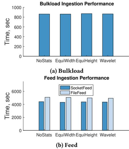
**Figure 2: Total execution time of ingesting 50M records (a) using a bulkload operation, which produces a single component, and (b) through a continuous data feed channel, which creates multiple LSM components. Both experiments are performed for 3 types of synopses (equi-width histograms, equi-height histograms and wavelets) and for a baseline case when the statistics collection is turned off (NoStats).**
