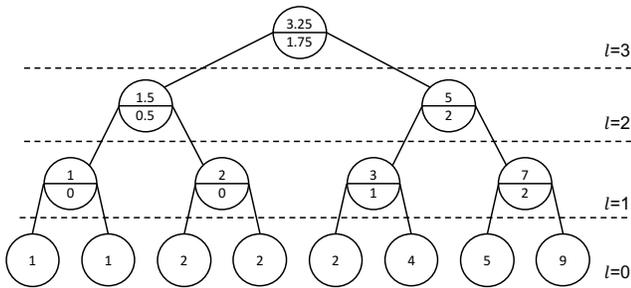
**Figure 11: Structure of error tree. Nodes on the lowest level ( $l = 3$ ) are comprised of the elements of prefix sum vector  $\mathcal{F}^+$ . Other nodes from the upper levels of the binary tree**
