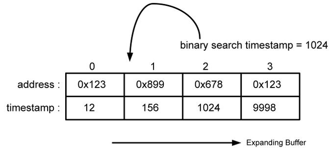
Fig. 12. Reducing the number of checks.
