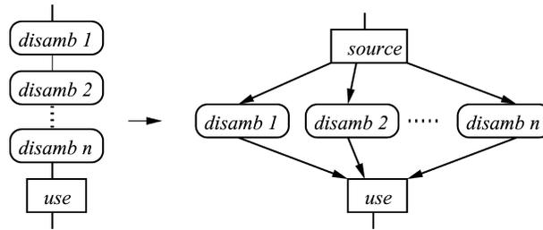
Fig. 10. Optimizing trace length by executing the disambiguation code of the correct store instruction.
