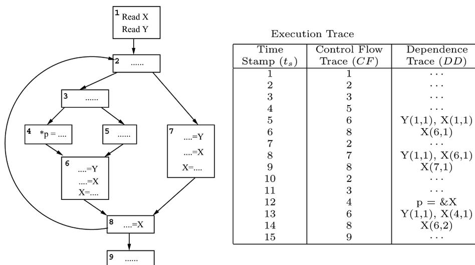
Fig. 15. Control flow and dependence trace.
