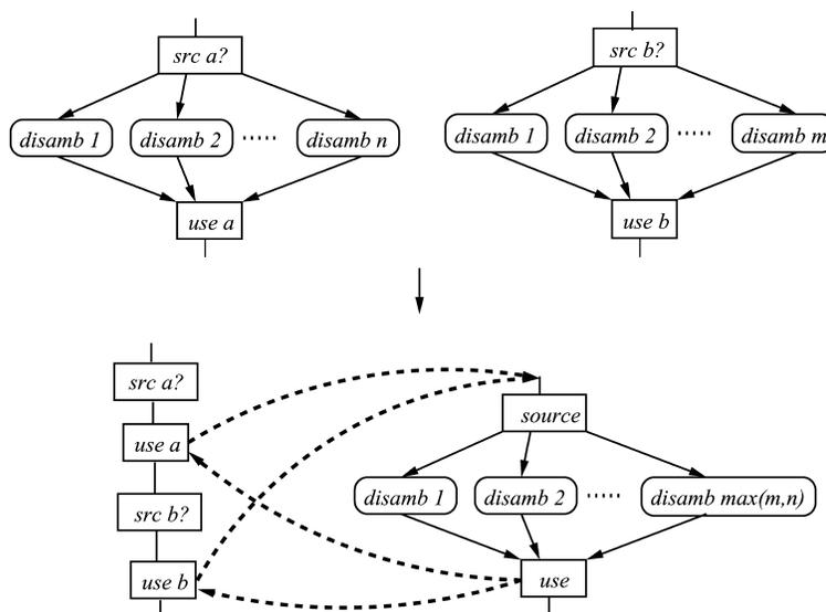
Fig. 11. Optimizing trace compressibility by executing a common piece of code.
