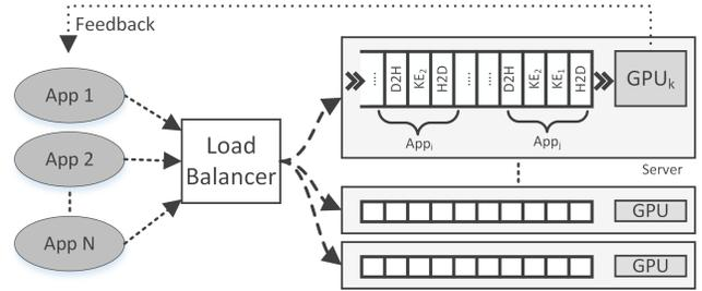
**Figure 3: Multi server GPU Sharing and per-server CUDA call queues in a typical cloud computing environment.**
