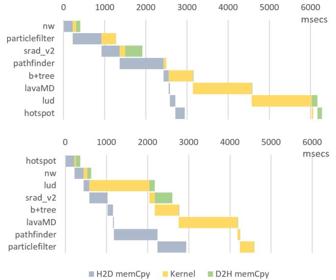
**Figure 2: (a) On the top, an overlapping example exploited on a subset of Rodinia applications using a random arrival ordering; and (b) On the bottom, a data transfer-aware re-ordering of the same subset.**
