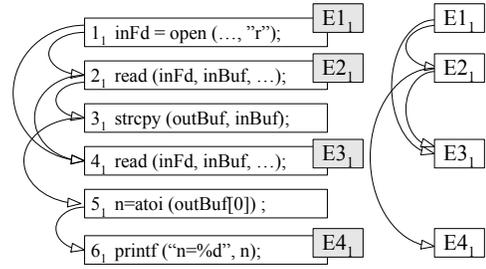
**Figure 3: An example of Dynamic Dependence Graph (DDG) and Event Dependence Graph (EDG).**
