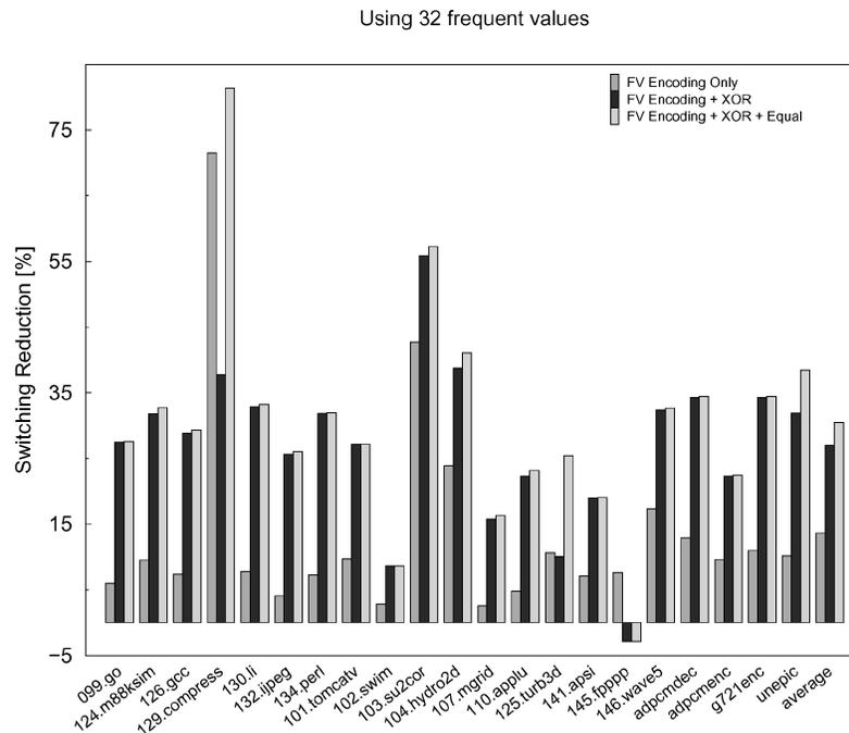
Fig. 10. Effectiveness of FV encoding and its enhancements.
