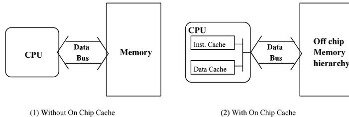
Fig. 18. Architecture models with and without on-chip caches.
