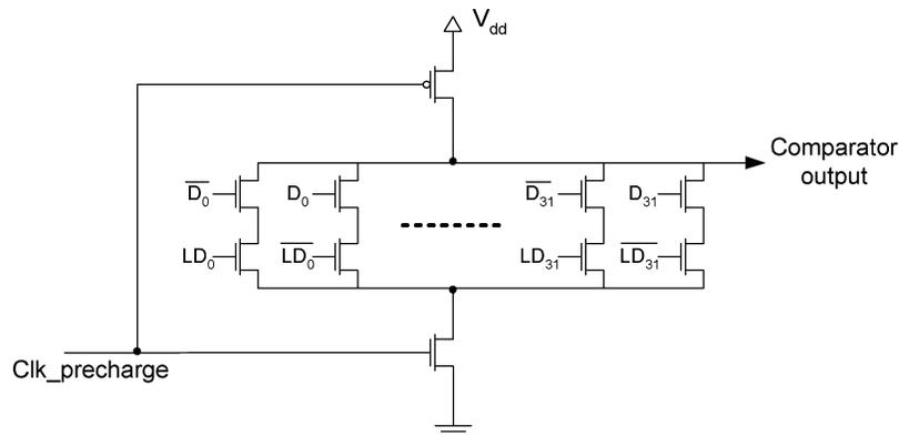
Fig. 21. Circuit for the comparator.  $D_i$  stands for the  $i$ th bit of the current data value.  $LD_i$  stands for the  $i$ th bit of the last data value.
