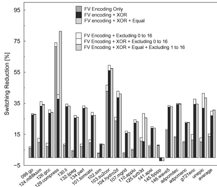
Fig. 11. Impact of excluding values on switching reduction.
