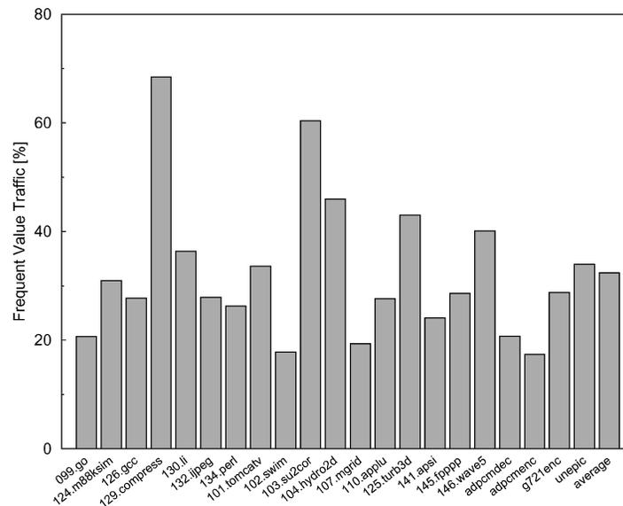
Fig. 1. Data bus traffic due to 32 frequent values.
