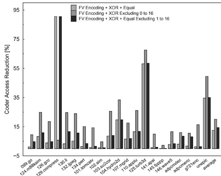
Fig. 12. Impact of excluding values on encoding/decoding operations.
