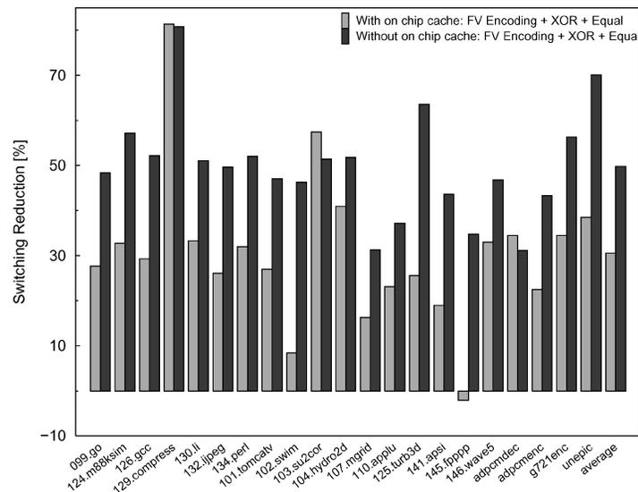
Fig. 19. FV encoding performance with on-chip cache versus without on-chip cache.
