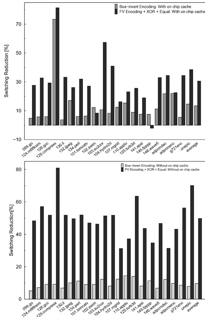
Fig. 28. Bus-invert versus enhanced FV encoding.
