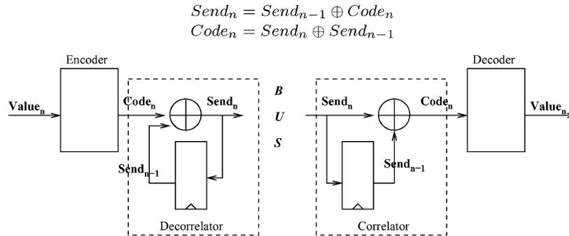
Fig. 4. Reducing switching by XORing values.
