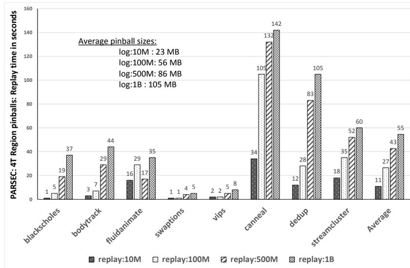
Figure 5.11: Replay times (wall clock) with pinballs for regions of varying sizes for some PARSEC benchmarks (‘native’ input).
