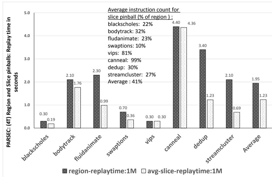
Figure 5.13: Execution slicing: average replay times (wall clock) for 10 slices for regions of length 1 million dynamic instructions: PARSEC ('native' input).
