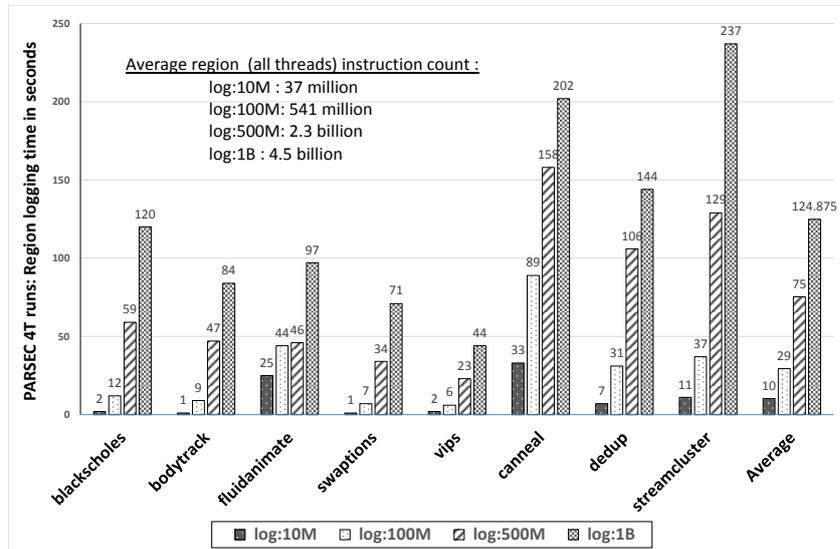
Figure 5.10: Logging times (wall clock) with regions of varying sizes for some PARSEC benchmarks (‘native’ input).
