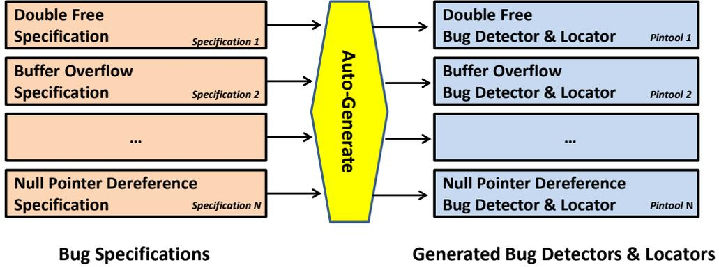
Figure 1.2: Extensibility via *bug specification* & *debugger generation*.
