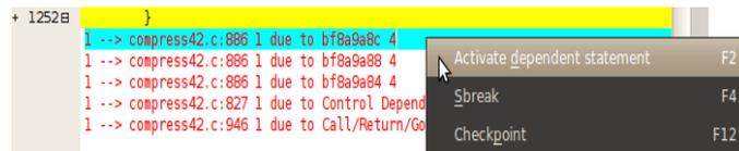
Figure 2.3: Slicing from the crash point.
