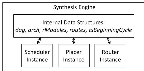
Figure 10. Synthesis engine contains an instance of a scheduler, placer and router, as well as internal data structures passed between synthesis steps.
