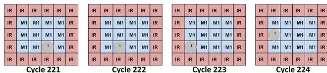
Figure 9. Illustration of droplet movement within a module.
