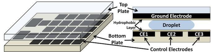
Figure 1. A DMFB with a 2D array of electrodes (left) and cross-sectional view of a DMFB (right).
