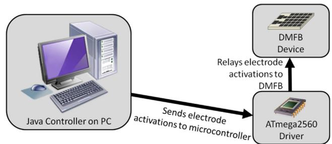
Fig. 27. Control software interface. An application written in Java and running on the host PC transmits a sequence of bit vectors representing electrode activations to an ATmega2560 microcontroller, which interfaces directly with the DMFB.
