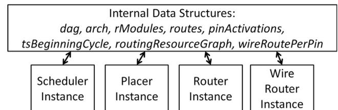
Fig. 9. The synthesis engine contains an instance of a scheduler, placer, (droplet) router, and (PCB) wire router, as well as internal data structures passed between synthesis steps.
