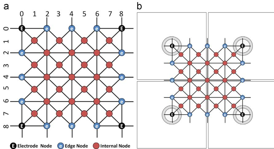
Fig. 10. (a) A routing graph tile used for PCB escape routing along with its planar coordinate system; (b) an overlaid routing graph on top of a  $2 \times 2$  electrode grid representing physical locations on the PCB.
