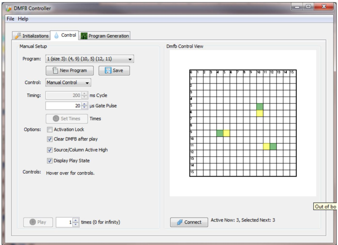
**Fig. 28.** Screenshot of the DMFB control software. The user can create and save manually-designed electrode activation sequences by clicking on cells in the “DMFB Control View” shown on the right; green cells are currently activated cells, while yellow represents cells that the user has selected for activation during the next cycle. (For interpretation of the references to color in this figure legend, the reader is referred to the web version of this article.)
