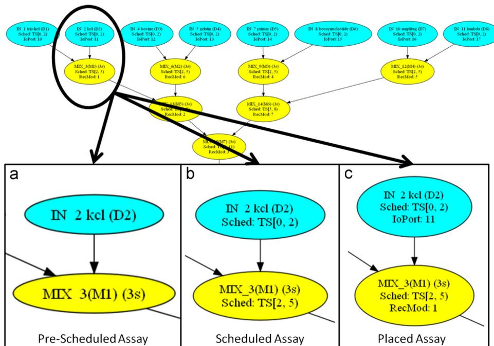
Fig. 13. GraphViz visualization for the assay prior to synthesis (a), scheduled (b), and placed (c). All text is legible in native output files.
