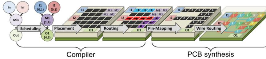
Fig. 3. The DMFB compiler consists of three stages: scheduling, placement, and droplet routing; the PCB synthesis flow adds pin-mapping and wire routing stages.
