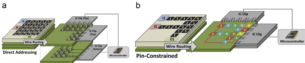
Fig. 5. A DMFB is typically mounted on top of a PCB that delivers signals provided by a microcontroller via one or more IC clips. The PCB may also include shift registers that latch the signals provided by the microcontroller. (a) A direct addressing DMFB presumably requires multiple PCB layers due to the large number of control signals that need to be routed; (b) a pin-constrained DMFB may require fewer PCB layers due to the reduced number of control inputs.
