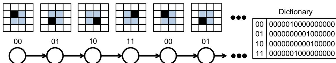
Fig. 29. Illustration of dictionary compression: redundant bit vectors are identified and put into a dictionary. Each state's output is now an index into the dictionary. The original Moore Machine had  $6 \times 16=98$  output bits; the compressed Moore Machine has a dictionary consisting of  $4 \times 16=64$  bits, while the state machine requires  $6 \times 2=12$  output bits, for a total of 76 bits.
