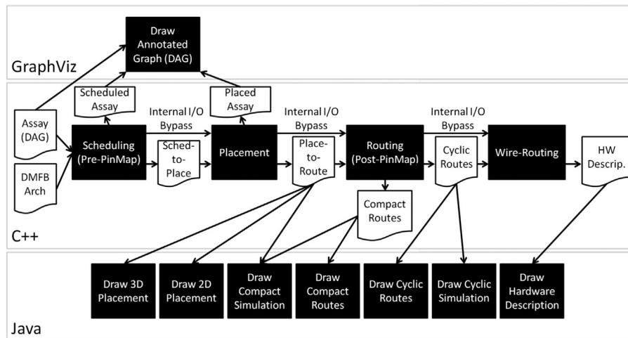
Fig. 8. Software architecture of the microfluidic framework, including compiler and synthesis algorithms (written in C++) and visualization tools.
