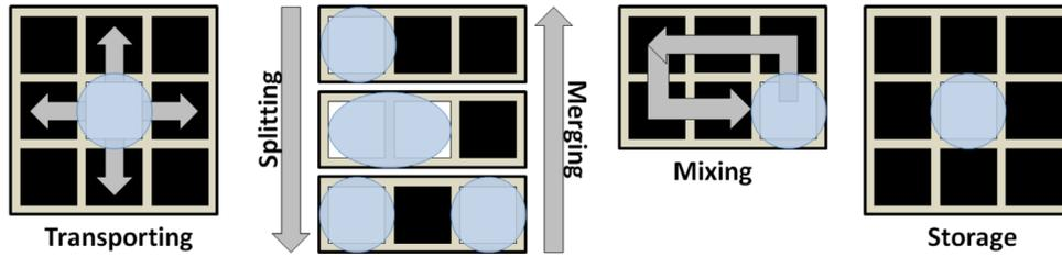
Fig. 2. The instruction set of a DMFB consists of five basic operations.
