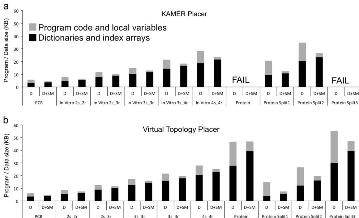
Fig. 30. Effectiveness of compression algorithms on program/data sizes using the (a) KAMER [2,44] and (b) virtual topology (VT) [21,22] placers.
