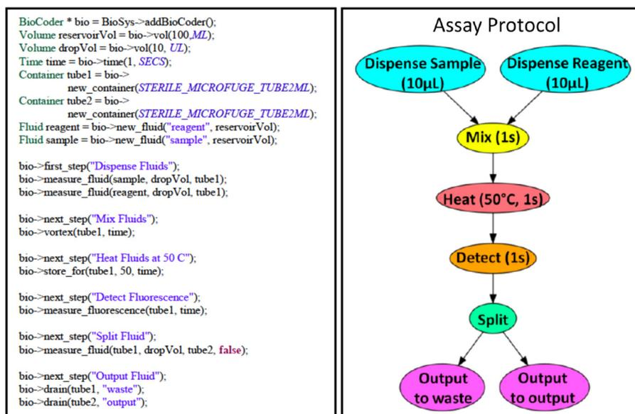
Fig. 7. A chemical reaction specified using our modified version of the BioCoder language (left) converted to a DAG (right).
