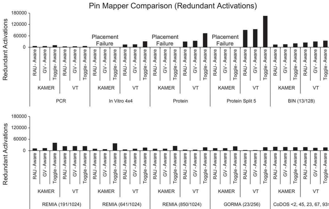
Fig. 24. The number of redundant activations (RAs) observed when using the RAU-Aware [36], GV-Aware [34], and Toggle-Aware [80] pin mappers, in conjunction with the KAMER and VT placers.
