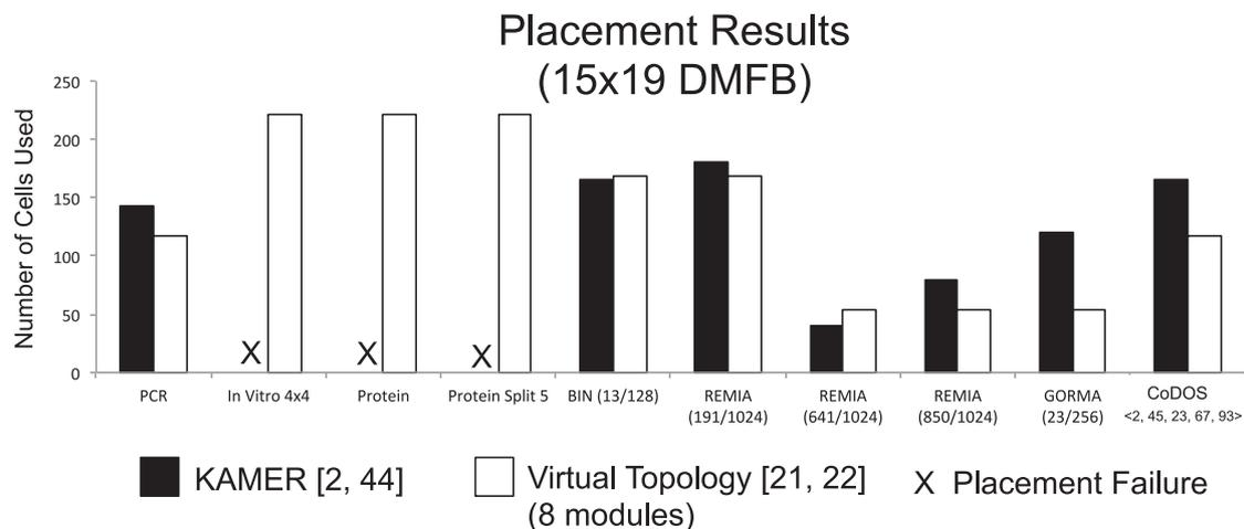
Fig. 19. Comparison of the KAMER [2,44] and Virtual Topology (VT) [21,22] placers on the 10 benchmark DAGs in Table 3.
