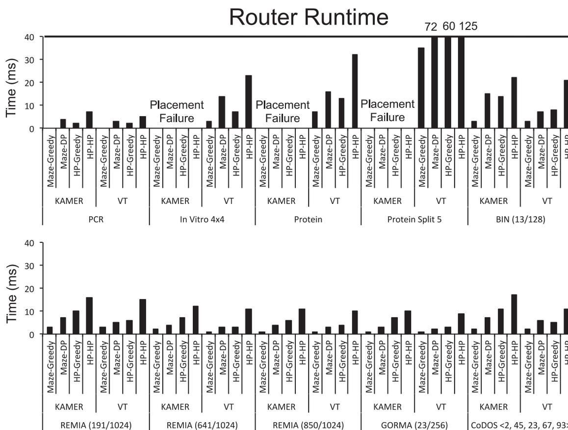
**Fig. 21.** Runtimes of the Maze-Greedy [64], Maze-DP [32,64], HP-Greedy [12,64], and HP-HP [12] routing algorithms across the 10 benchmarks from Table 3 using the KAMER and Virtual Topology (VT) placement heuristics.
