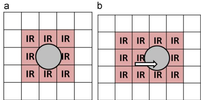
Fig. 12. The interference region of a droplet (a) at rest and (b) moving. If any other droplet enters the interference region, the two will inadvertently merge.
