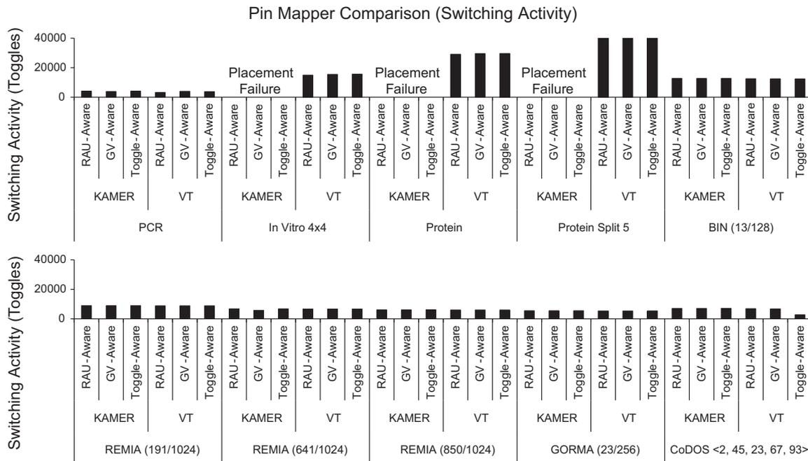
Fig. 25. The switching activities (toggles) observed when using the RAU-Aware [36], GV-Aware [34], and Toggle-Aware [80] pin mappers, in conjunction with the KAMER and VT placers.
