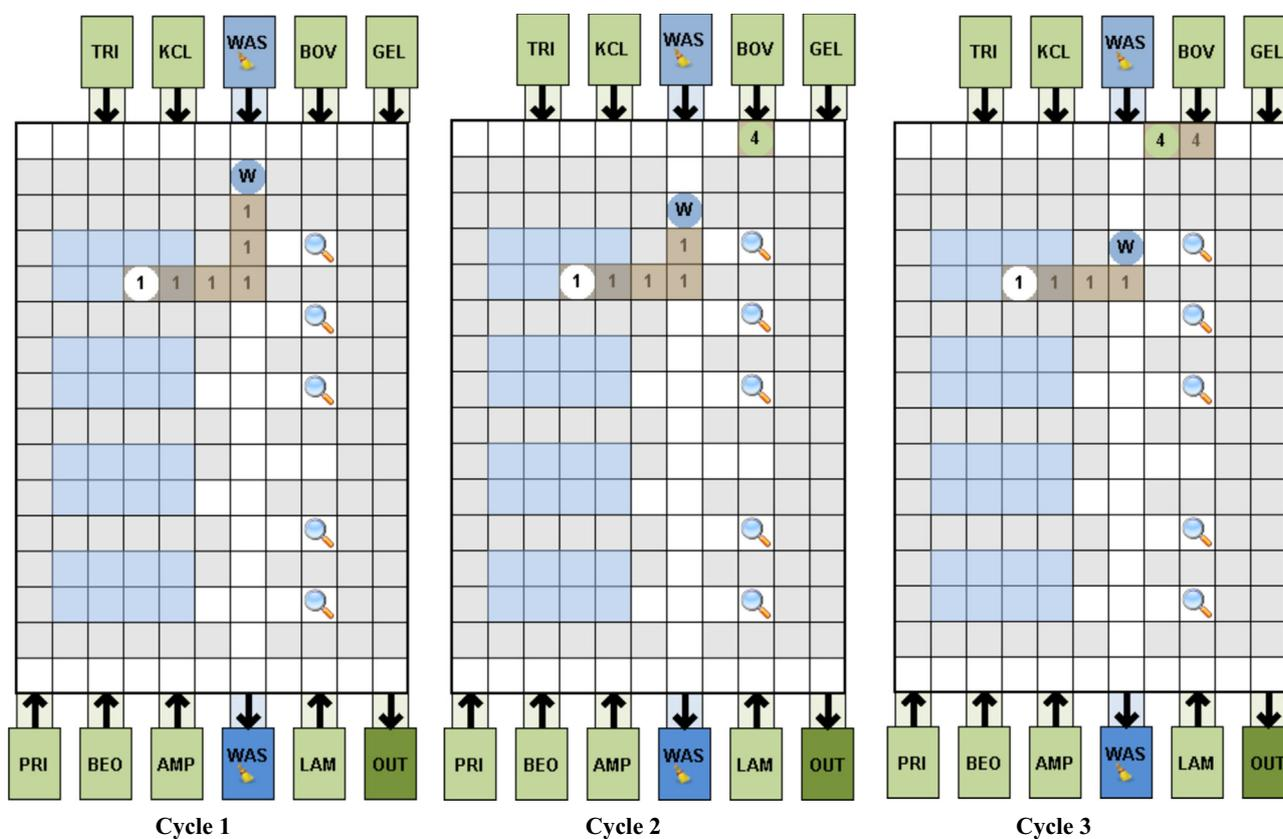
Fig. 17. Three cycles of an assay showing dirty cells (brown cells) marked by the ID of the droplet which made it dirty. Wash droplets (blue, labeled 'W') have specific input and output reservoirs (blue I/O ports with broom labeled 'WAS') and clean dirty cells (removing the brown shading). (For interpretation of the references to color in this figure legend, the reader is referred to the web version of this article.)
