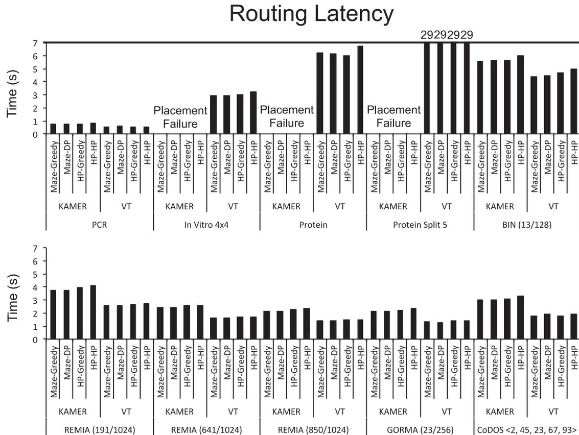
**Fig. 20.** Performance comparison of the Maze-Greedy [64], Maze-DP [32,64], HP-Greedy [12,64], and HP-HP [12] routing algorithms across the 10 benchmarks from Table 3 using the KAMER and Virtual Topology (VT) placement heuristics.
