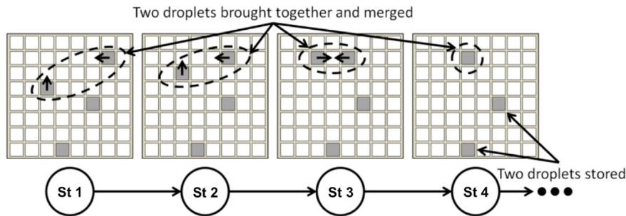
Fig. 4. The output of a DMFB compiler is a linear state machine in which each state specifies a subset of electrodes to activate at a given time.
