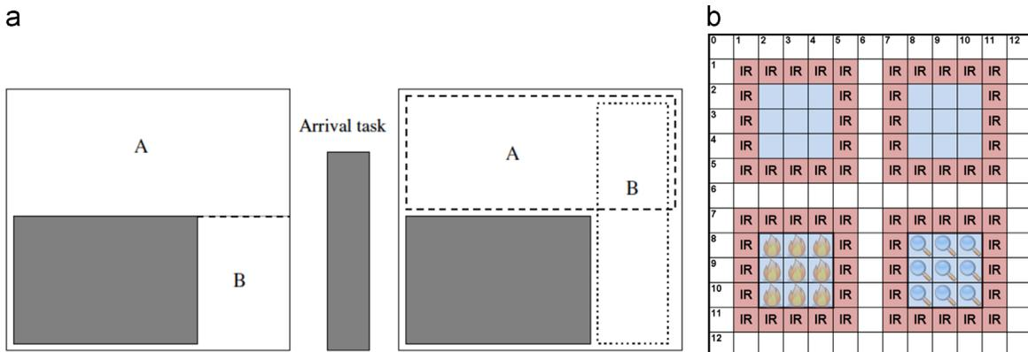
Fig. 11. (a) Illustration of the way that the KAMER algorithm represents free-space on the chip using (possibly overlapping) maximum empty rectangles (MERs) [2,44]. (b) Illustration of a 4-module virtual topology [21,22], where one of the four modules has a heater and another has a detector.
