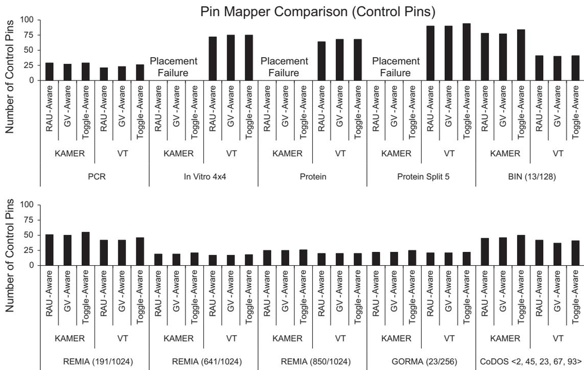
Fig. 23. The number of control pins obtained using the RAU-Aware [36], GV-Aware [34], and Toggle-Aware [80] pin mappers, with KAMER and VT placers.
