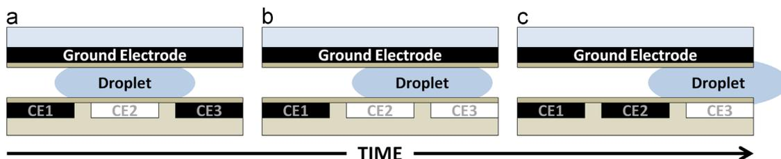
Fig. 1. A DMFB is a 2-dimensional planar array of electrodes; (b) a cross-sectional view of a DMFB, showing the ground electrode on top and a droplet sandwiched in-between; (c) illustration of droplet transport by a sequence of activated electrodes (activation is shown in white).
