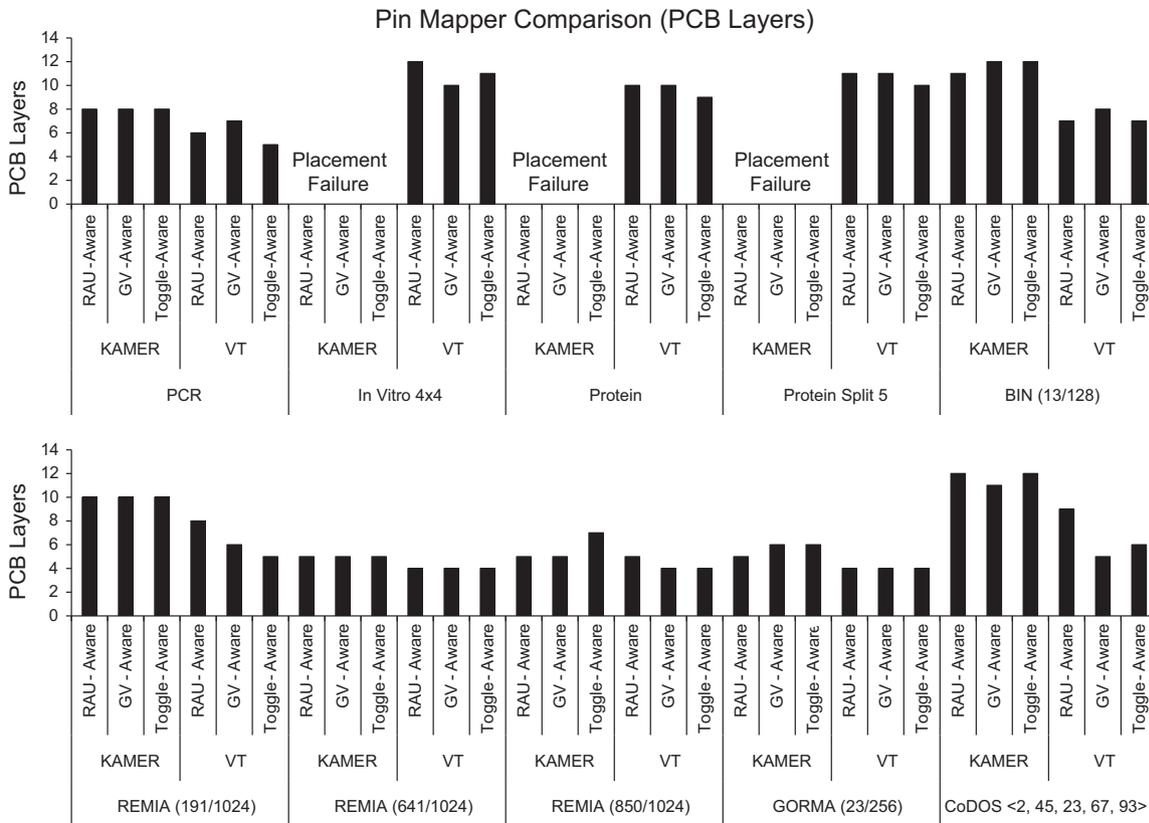
Fig. 22. The number of PCB layers obtained using the RAU-Aware [36], GV-Aware [34], and Toggle-Aware [80] pin mappers, with KAMER and VT placers.
