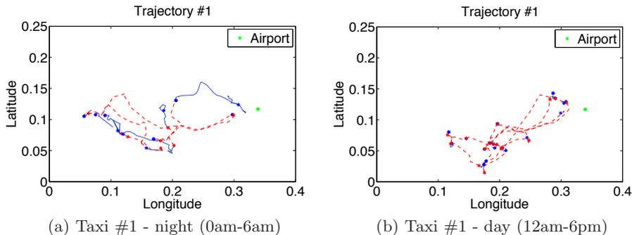
**Fig. 2.** Night vs day trajectories of the same taxi: (a) during the night, the blue (=‘empty’) trail is linear-like, probably going to the airport (green dot), or to taxi plazas; (b) during the daytime, the blue (empty) trail is point-like, due to wandering behavior, to find nearby passengers. In all cases, the red (=‘full’) trails are linear-like. Note that we anonymize latitude and longitude information due to privacy concerns.
