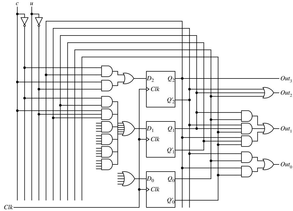
3. Use a 4-bit up/down counter with parallel load to design a counter circuit that counts the following sequence repeatedly.
