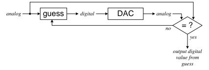
Given an analog input signal, a guess circuit guesses what the digital value should be. This digital value is inputted into a DAC. The resulting analog signal is compared with the original analog signal. If they are equal, then the guess digital signal is outputted. Otherwise the guessing continues. The guessing can be similar to a binary search algorithm.
