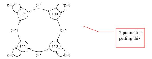
2. Synthesize a circuit that will count the following sequence using only <u>one</u> type of flip-flops:
