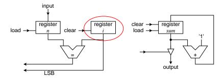
c) Can't compare  $(i \mod 2) == 0$ . Need a mux and input a '0'.
