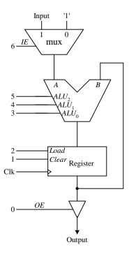
Test the circuit with the counting program that outputs the numbers from 0 to 9 as presented in class.
