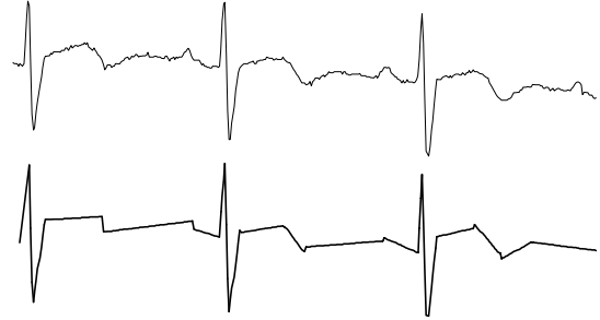
Figure 8. An example of a time series with its piecewise linear representation
