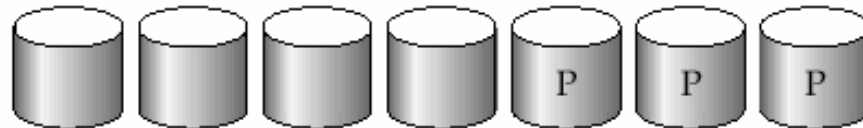
(c) RAID 2: memory-style error-correcting codes
