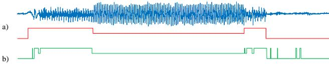
Figure 7: PAMAP test data (Blue) with annotations (Red). The bars with the same height represent the same types of activities. Despite confusions between activities in some regions, our algorithm (Green) correctly found almost all instances of walking and standing.
