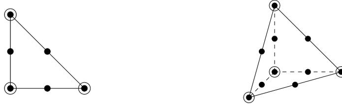
Figure 4:  $(P_2, P_1)$  Taylor-Hood elements for 2D and 3D. The filled circles (●) are velocity degrees of freedom and hollow circles (○) are pressure degrees of freedom.
