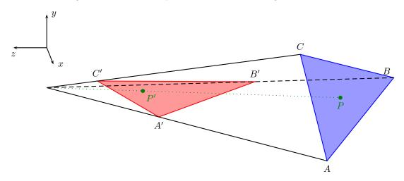
2. Transform from A,B,C,P to A',B',C',P' by homogeneous matrix  ${\bf M}.$
