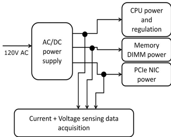
Fig. 9. Power measurement configuration.
