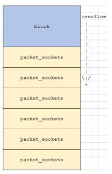
packet\_sock-xmit is called when a user sends a packet via the socket. If we overwrite this function pointer and make it point to the executable memory region, for example, the commit creds (prepare kernel cred(0)).
