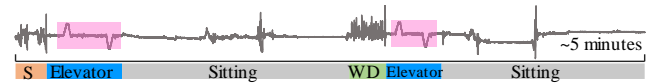
Fig. 4. The hip-mounted X-axis acceleration of a graduate student standing, using elevator, sitting, walking down stairs, using elevator and sitting again. The data is real but edited for visual brevity [18].
