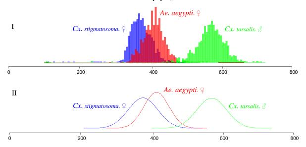
Figure 1: I) Histograms of wingbeat frequencies of three species of insects, *Cx. stigmatosoma*  $\bigcirc$ , *Ae. aegypti.*  $\bigcirc$ , and *Cx. tarsalis.*  $\bigcirc$ . Each histogram is derived based on 1,000 wingbeat sound snippets. II) Gaussian curves that fit the wingbeat frequency histograms
