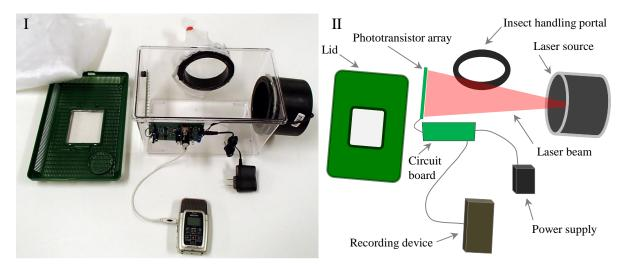
Figure 2: I) One of the cages used to gather data for this project. II) A logical version of the setup with the components annotated
