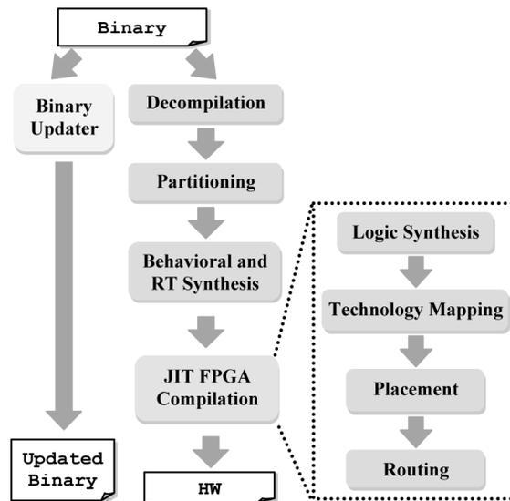
Fig. 6. ROCCAD on-chip CAD tool chain.
