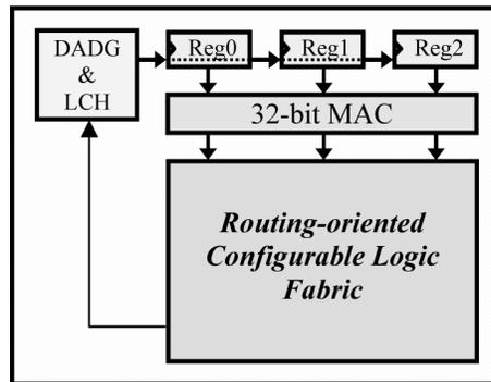
Fig. 4. A warp-oriented field programmable gate array (W-FPGA).
