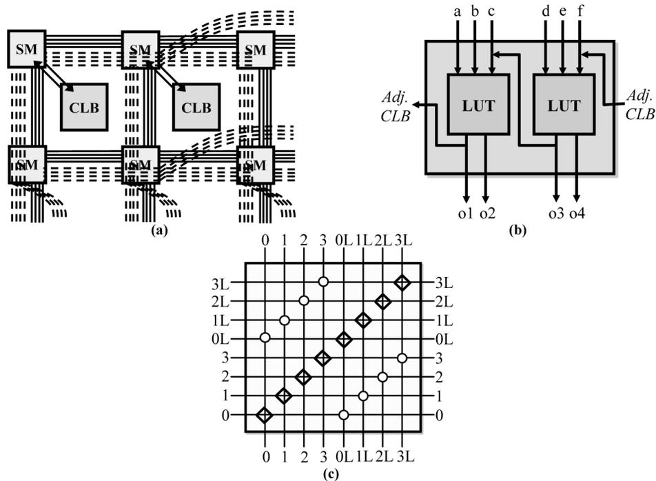
Fig. 5. (a) A routing-oriented configurable logic fabric, (b) combinational logic block, and (c) switch matrix architecture.
