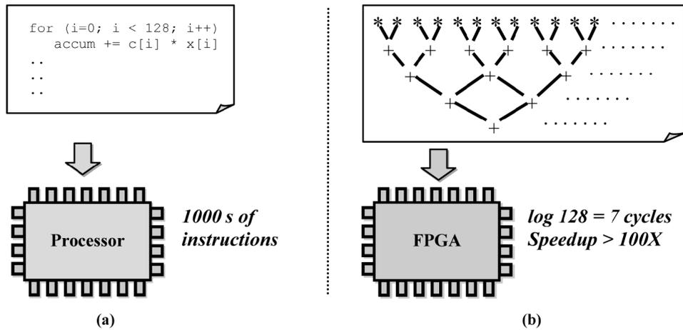
Fig. 2. FIR filter implemented in (a) software on a microprocessor and (b) hardware on an FPGA.
