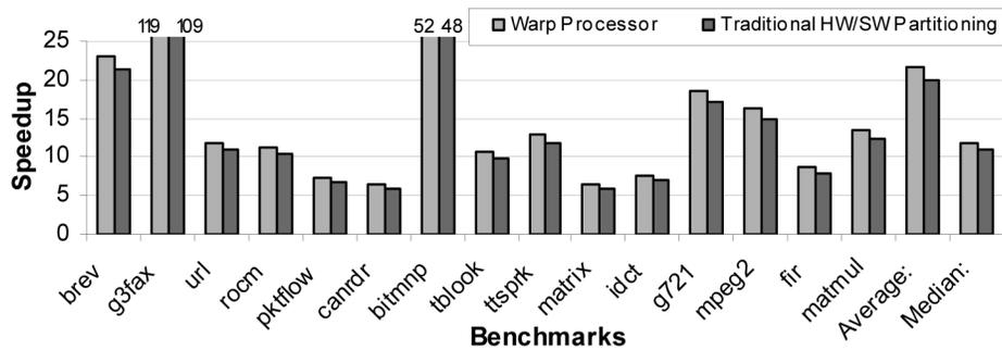
Fig. 7. Critical region speedup of a single critical region implemented using warp processors and traditional hardware/software partitioning, targeting an FPGA for NetBench, MediaBench, EEMBC, and Powerstone benchmark applications.
