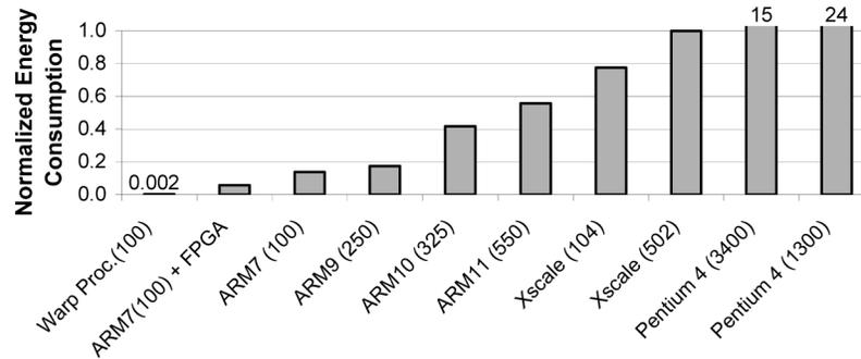
Fig. 12. Average overall energy consumption of NetBench, MediaBench, EEMBC, and Powerstone benchmark applications using various processors normalized to the XScale processor at 502 MHz (processor frequency reported in megahertz).
