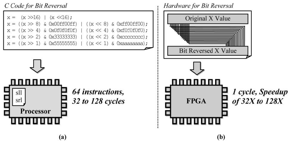
Fig. 1. A comparison of a bit reversal in (a) software on a microprocessor and (b) hardware on an FPGA.
