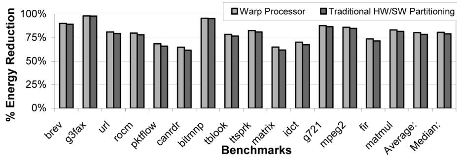
Fig. 8. Critical region energy reduction of a single critical region implemented using warp processors and traditional hardware/software partitioning, targeting an FPGA for NetBench, MediaBench, EEMBC, and Powerstone benchmark applications.
