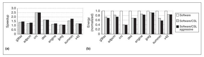
Figure 2. Estimated results for MIPS platform: speedup (a) and energy consumption (b) for partitioned examples.
