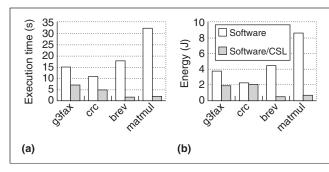
Figure 3. Measured results for Triscend E5 platform: execution times (a) and energy consumption (b) for the software and partitioned examples.
