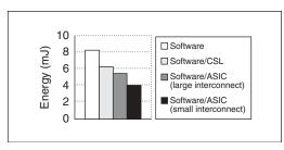
Figure 6. Comparison of estimated energy savings for MIPS-CSL design and MIPS-based ASIC design.
