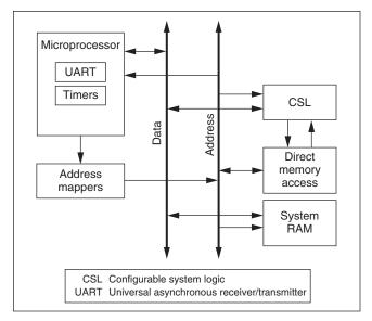
Figure 1. Triscend E5 single-chip architecture.
