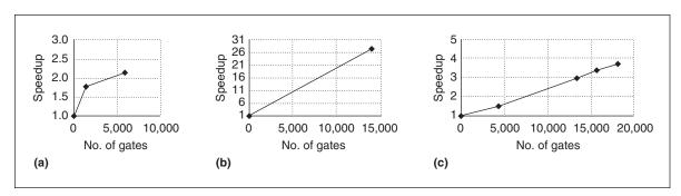
Figure 5. Relationship between size and speedup for several MediaBench examples: G721 (a); adpcm (b); and Pegwit (c).
