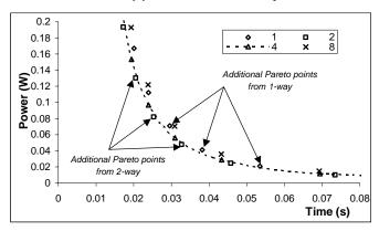
Figure 2: Power vs. time for the g3fax example. The configurable associativity yields additional Pareto points.
