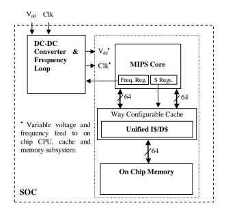
for both instruction and data. For simplicity in this work, our cache's ways could only be disabled or used for both instruction and data, but the methods can be applied to cache's with greater or lesser configurability.
