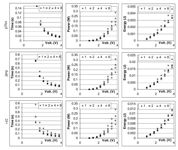
Figure 3: Time, power and energy data for the three examples.
