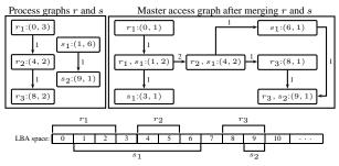
Figure 4: **Building the master access graph.** Vertices are defined by (start LBA, size of request). Since vertices  $r_1$  and  $s_1$  have overlapping LBAs,  $r_1$  is split into two vertices in the master access graph, one with size 1 and the other with the overlapping  $s_1$  blocks, starting at LBA 1 with size 2.
