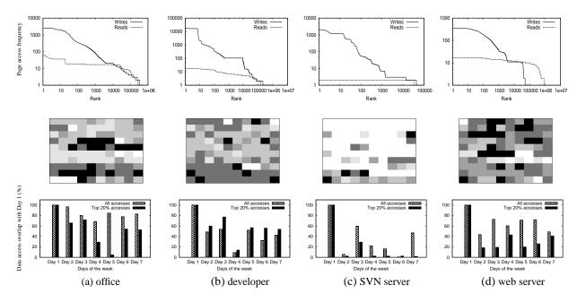
Figure 1: Rank-frequency, heatmap, and working-set plots for week-long traces from four different systems. The heatmaps (middle row) depict frequency of accesses in various physical regions of the disk, each cell representing a region. Six normalized, exponentially-increasing heat levels are used in each heatmap where darker cells represent higher frequency of accesses to the region. Disk regions are mapped to cells in row-major order.
