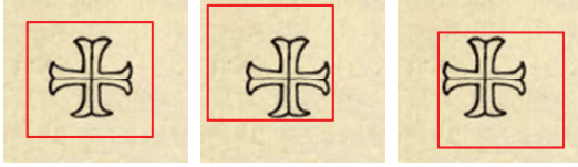
Figure 4. The distance measure we use is offset-invariant, so the distance between any pair of windows, left , center or right above, is exactly zero. This simple fact can be exploited to greatly reduce the search space of motif discovery. Since a pattern from another book that matches one of the above with a distance X must match all with distance X , we only need to include any one of the above in our search.
