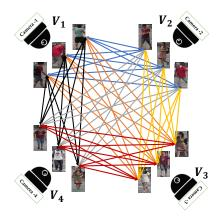
Figure 2: This figure demonstrates representation of a camera network with four cameras as a k-partite graph with k=4.
