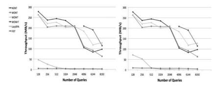
Fig. 6. Hardware vs. software performance with an increasing number of queries for streams of 5 MB (left) and 50 MB (right)
