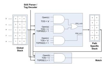
Fig. 2. Optimized hardware mapping for the matching of XPath a/c/a/c/b. Stack contents reflect on a macthed state of the expression.
